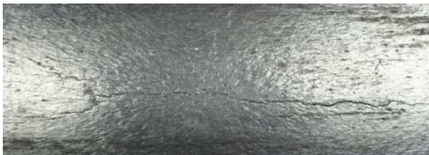
Figure 4. Cracks with longitudinal chipping in the rear zinc plate
