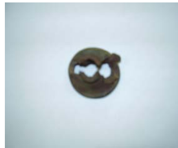
Figure 5. Three entry holes in the lid instead of one after the explosion of 18 g charge with a composite liner (W – Cu – Pb)
