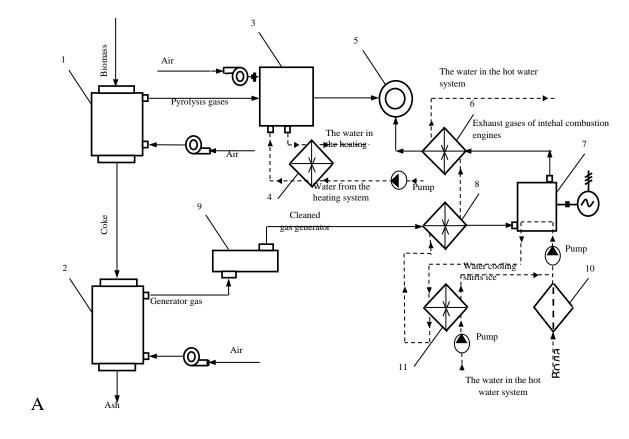
1-pyrolyzer, 2- gasifier; 3- hot water boiler; 4- the heat exchanger of the heating system; 5- chimney; 6- the cooler exhaust gases; 7- internal combustion engine; 8- cooler generator gas; 9- gas purification; 10- chemical water treatment; 11- cooler shirts engine.
