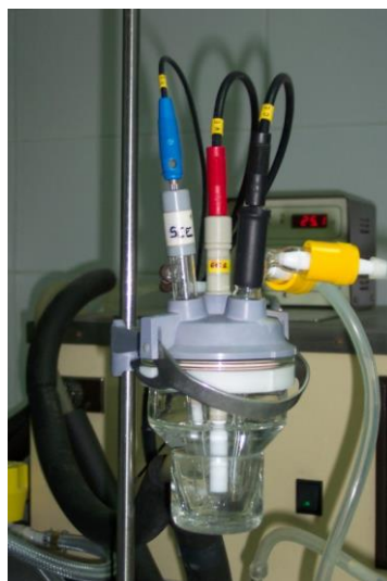
Figure 1. Conventional electrochemical cell of three electrodes.
