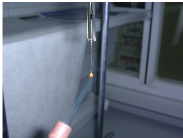
Figure 2. Flame annealing procedure of a polyfaceted gold bead.
