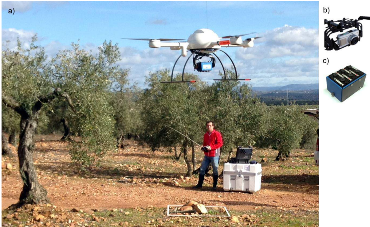
Figure 2. The quadcopter UAV, model md4-1000, taking off in one of the studied fields (a) and the sensors used in this investigation: the visible-light camera (b) and the multispectral camera (c).
