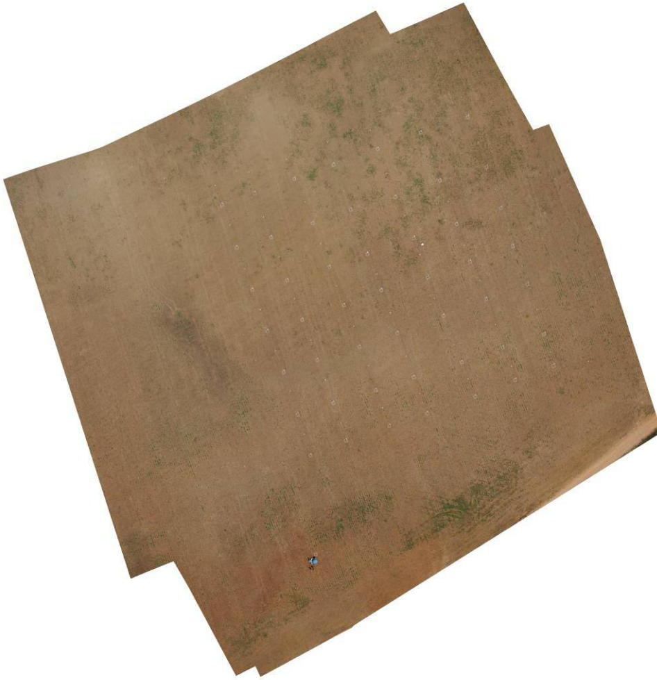
Figure 6. Ortho-mosaic of the whole experimental field. Composed from six individual images taken by the still RGB camera at 100 meters altitude.
