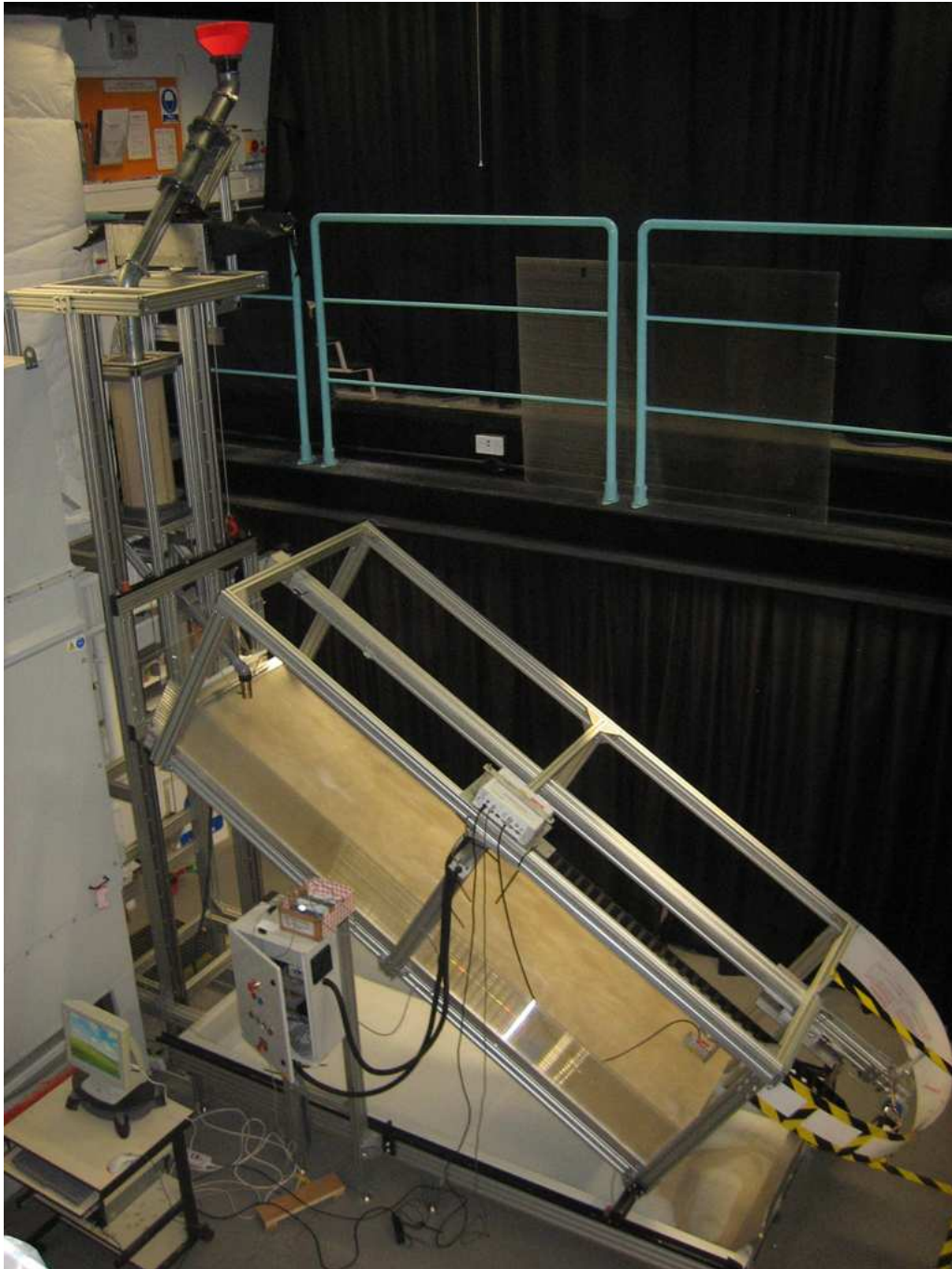
Figure 8.1: Photograph of the experimental configuration. The rough inclined plane is supported by an aluminium structure.
