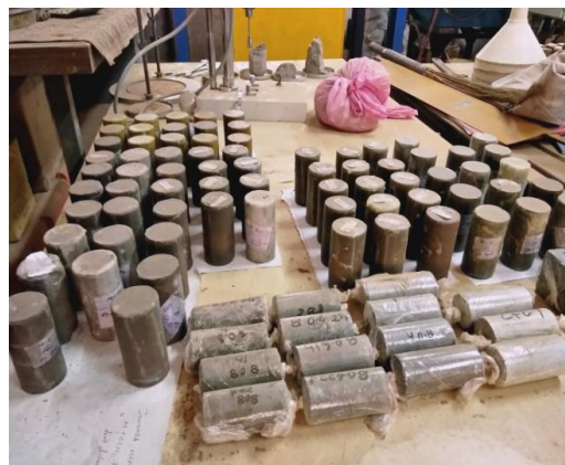
Fig 3.6. UCS samples coated with wax.
