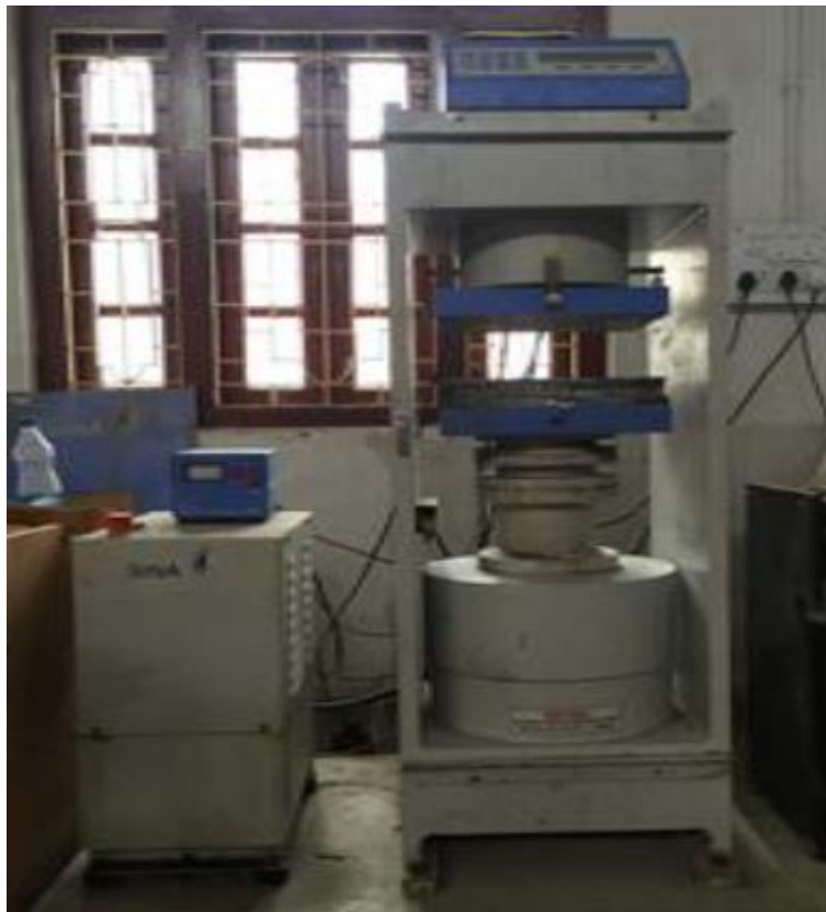
Fig 3.8 Compressive testing machine of paver block
