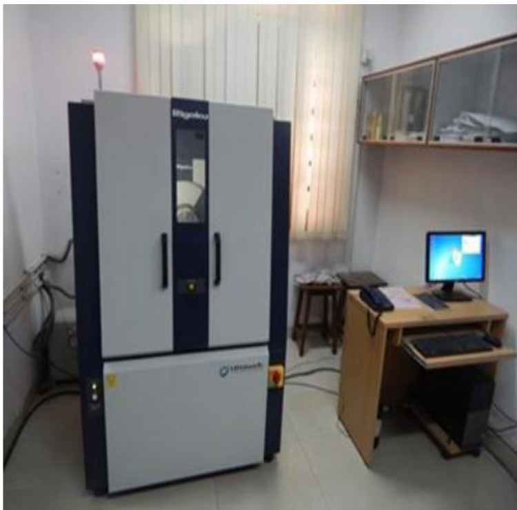
Fig 3.11 Multipurpose X-ray diffraction system (Rigaku ULTIMA IV)
