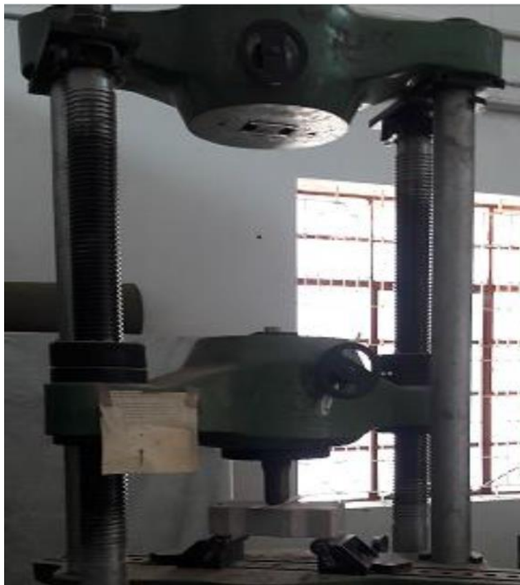
Fig 3.9 Flexural strength test conducted by using Universal Testing Machine
