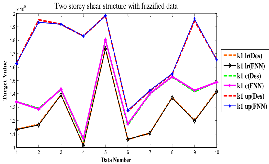
Figure 3.9(a): Comparison between desired and FNN values of \hat{k}_1 for a double storey shear structure
