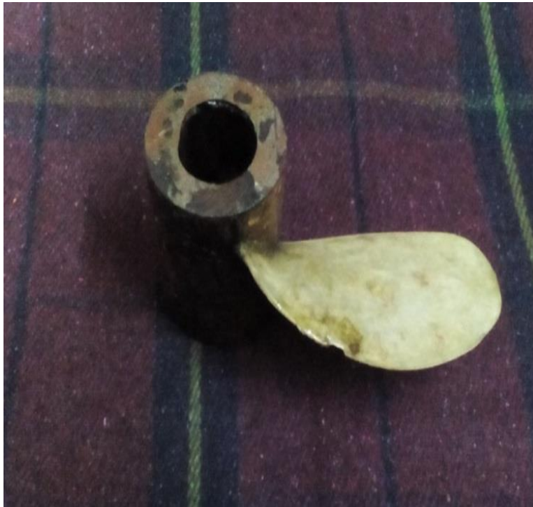
Figure 4.51: Fabricated model of E-glass epoxy blade
