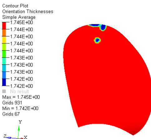
Figure 5.20: Contour plot for orientation thickness (mm) E-glass epoxy blade for ply angle 45^\circ
