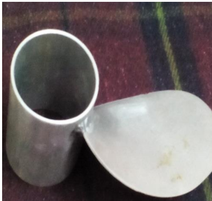
Figure 4.43: Fabricated model of Aluminium single bladed propeller
