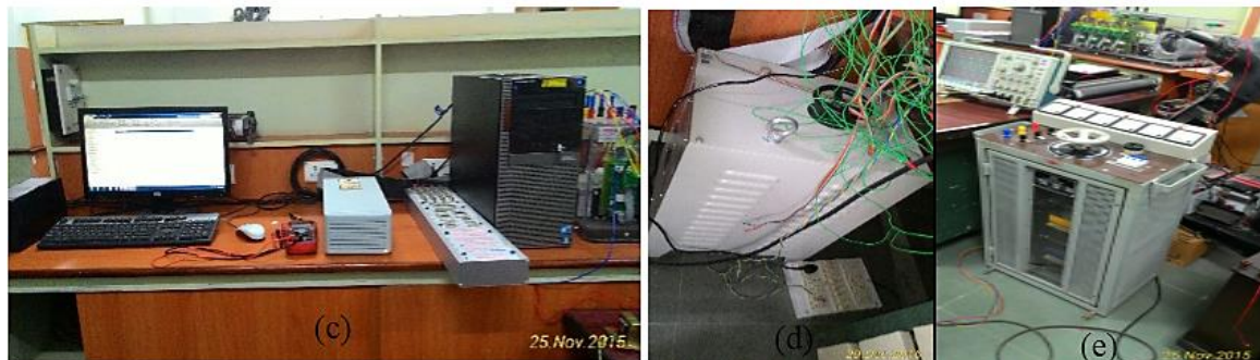
Fig. 3.20 Photograph of experimental set-up (a) solar panels (b) host computer with dSPACE R&D board and connector panel (c) auto transformer (d) interfacing inductor
