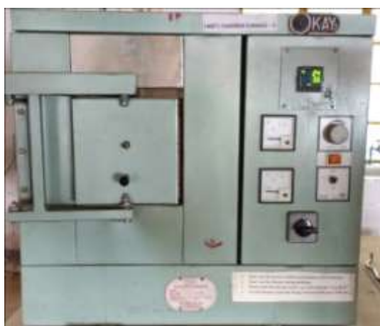
Figure 5. Image of the electric furnace used for calcinations
