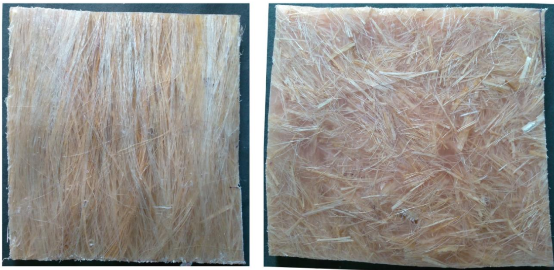
Figure 4.6: Fabricated composite sheets by hand lay-up technique
