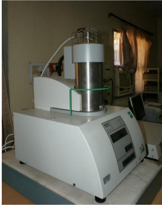
Figure 4.15: Experimental set up of NETZSCH STA 449 C Jupiter®
