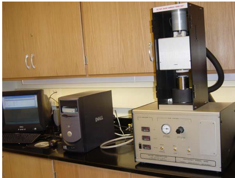
Figure 4.13: Experimental set up of Unitherm™ 2022
