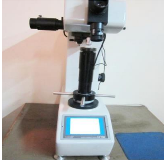
Figure 4.11: Experimental set up for micro-hardness test
