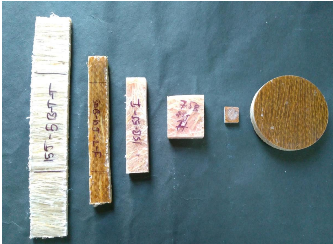
Figure 4.7: Composite specimens as per ASTM standards
