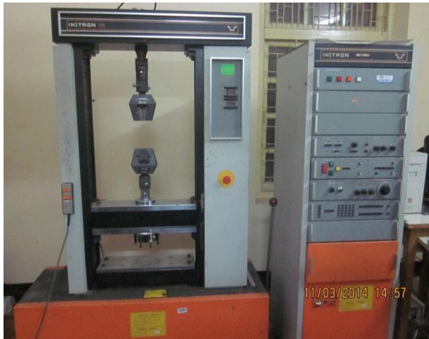
Figure 4.9 Universal testing machine (Instron 1195)
