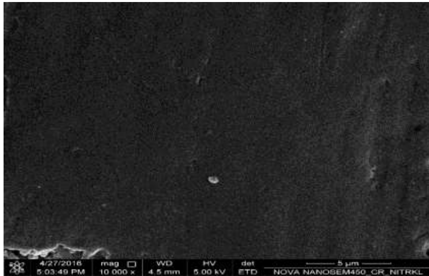
Figure. 17. Micrographs of PP wax at 10000 magnification
