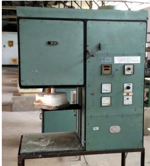
Figure 3.7: High Temperature Raising Hearth Furnace
