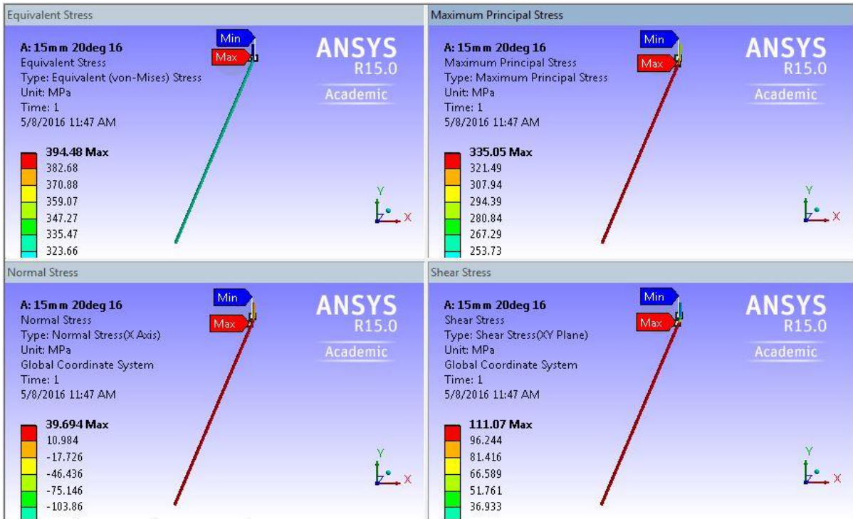
Figure 5-12 Contact stresses result of 15mm wire inclined at 20deg applied tension 16N
