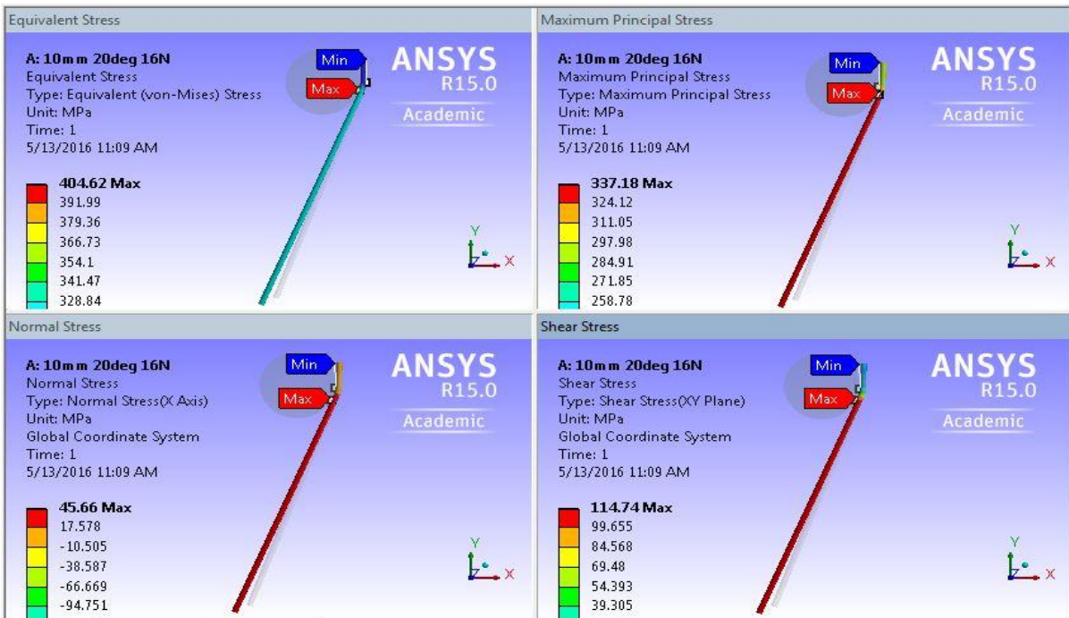
Figure 5-8 Contact stresses result of 10mm wire inclined at 20deg applied tension 16N
