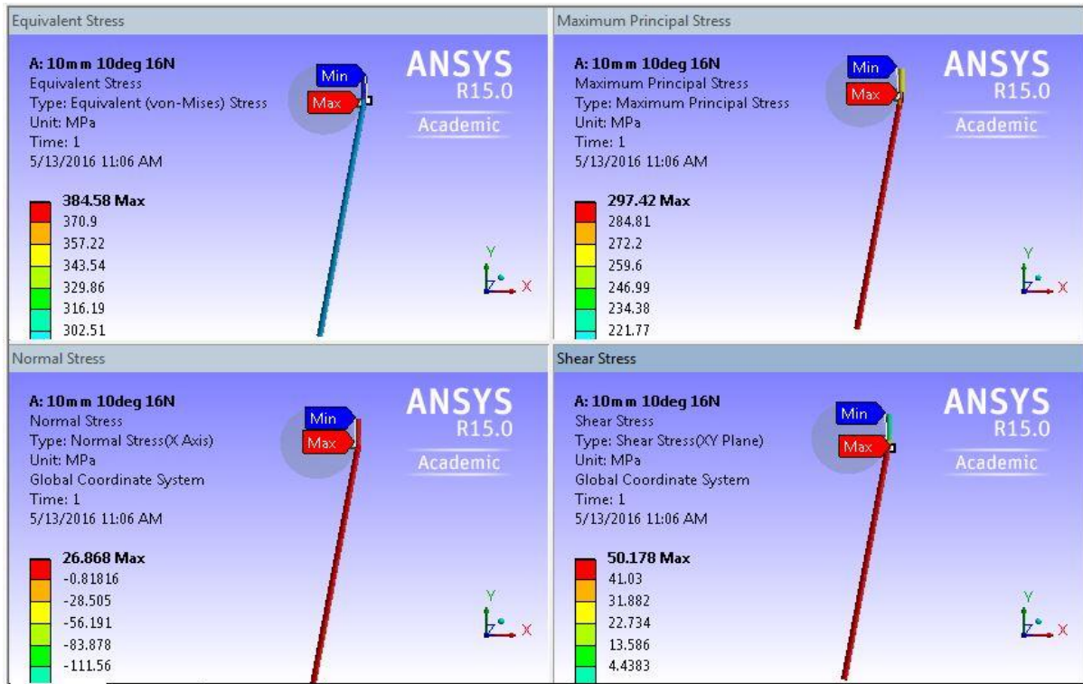
Figure 5-6 Contact stresses result of 10mm wire inclined at 10deg applied tension 16N
