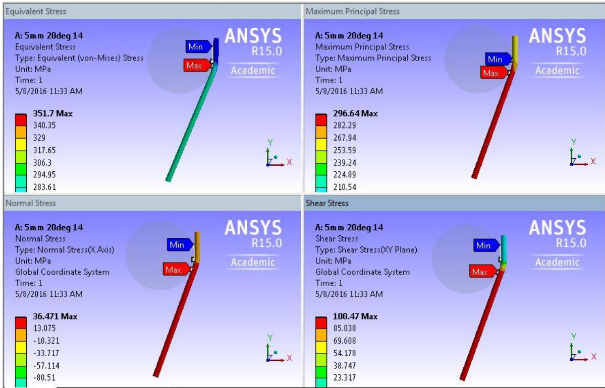
Figure 5-3 Contact stresses result of 5mm wire inclined at 20deg applied tension 14N
