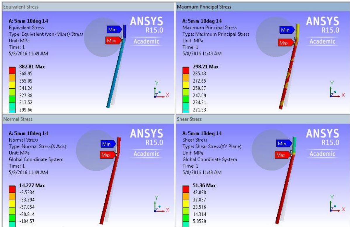
Figure 5-1 Contact stresses result of 5mm wire inclined at 10deg applied tension 14N
