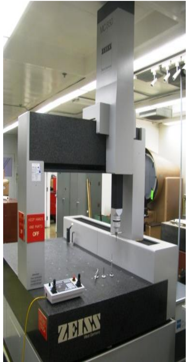
Figure 4-6 ZEISS MC 850 Coordinate measuring machine for angular measurement
