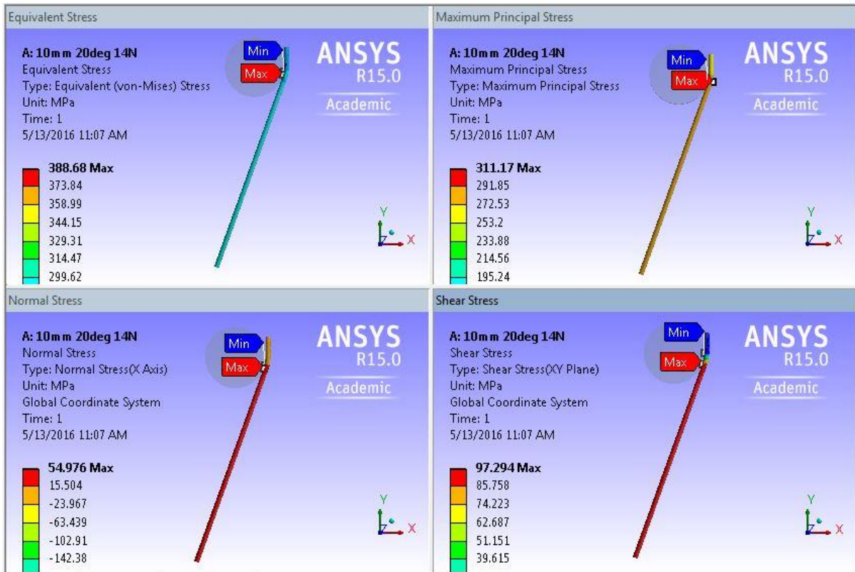
Figure 5-7 Contact stresses result of 10mm wire inclined at 20deg applied tension 14N
