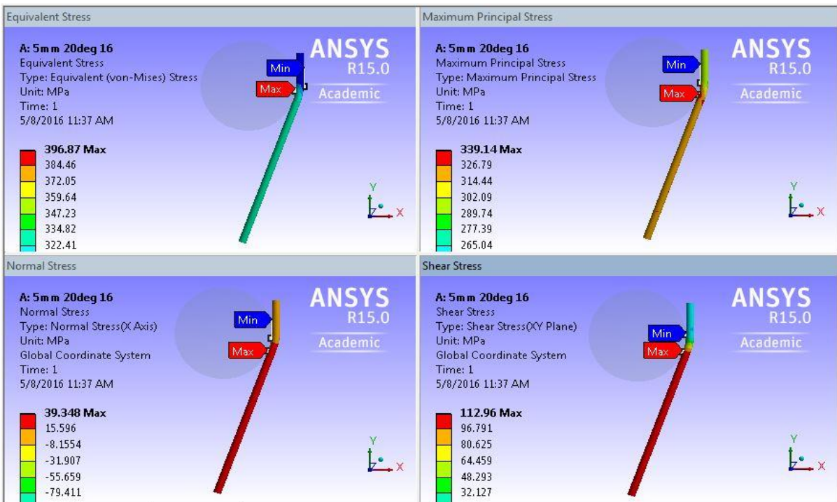
Figure 5-4 Contact stresses result of 5mm wire inclined at 20deg applied tension 16N
