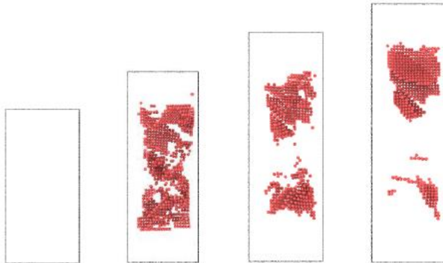
Fig.4.1.2.2.3(a) Atomic configuration of Nano-copper at points O, D, E, F corresponding to the stress-strain curve. Fig.4.1.2.2.3(b) The perfect fcc atoms and surface atoms are removed to show the stacking fault generated by the \{1\ 1\ 1\}/\{1\ 1\ 2\} partial slip.
