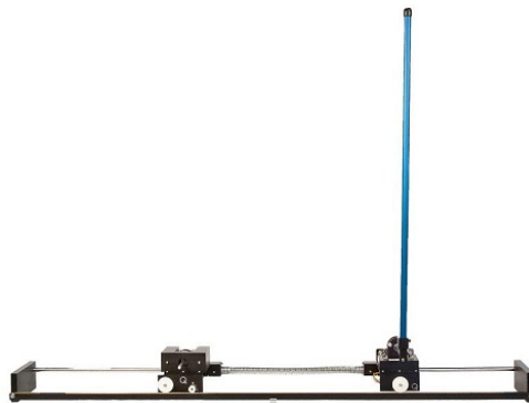
Figure 1.1: Cart-Inverted Pendulum System
