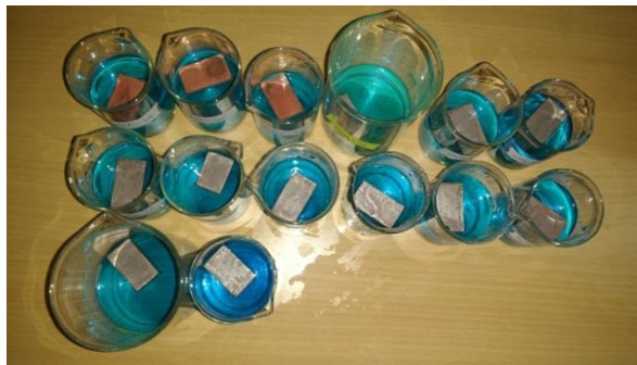
Figure 3.5: Parts immersed into various electroless baths.
