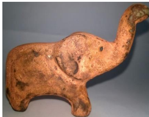
Figure 4.3: Elephant made by ABS after electroless Cu coating.
