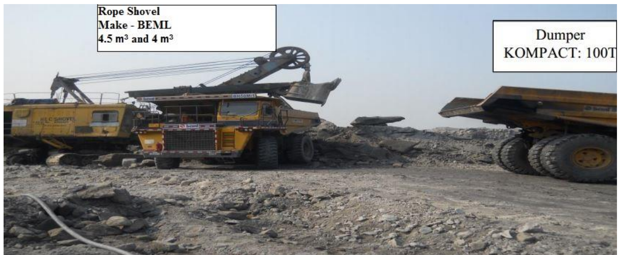
Figure 27 - Working of Rope Shovel and Dumper
