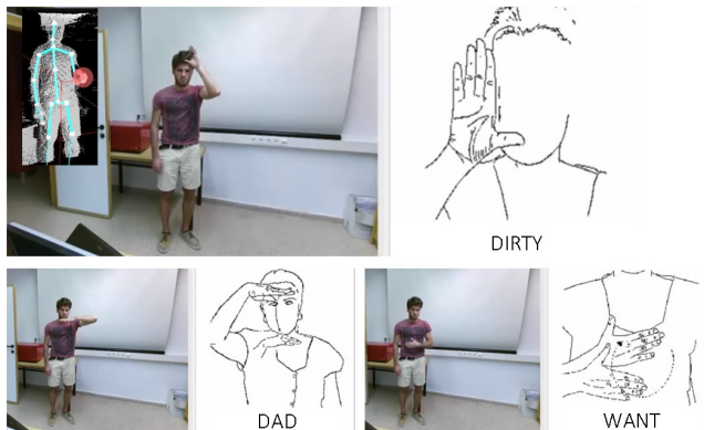
Fig. 4. Example of a user performing body and hand gestures in front of the robotic platform. The proposed system can recognize a subset of Schaefer's gestures for human-computer communication. Top left: shows the 3D skeleton and tracked 3D joints used for recognizing the gesture performed. On the right part of each sub-image, we can see the gesture recognized by the system.
