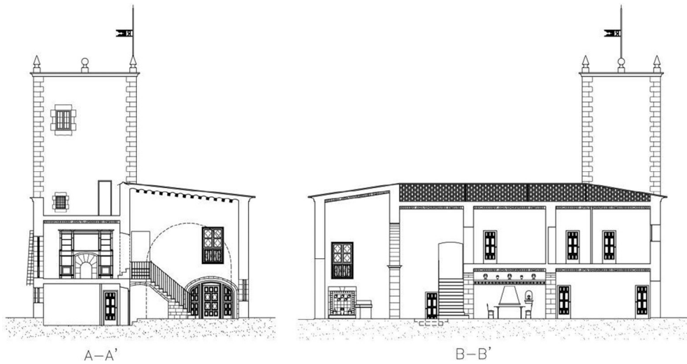
Figure 8: Left. A-A' cross section. We can see the entrance door to the tower at the first floor and the two levels hall with the big arch. Right. B-B' longitudinal section, a house global vision.
