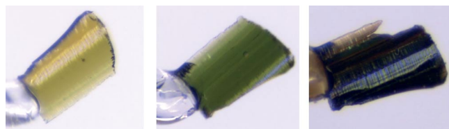
Figure 1. Photos of a single crystal of bp4pc·2H 2 O at room temperature (left), heated at 140 °C (middle), and heated at 160 °C (right).
