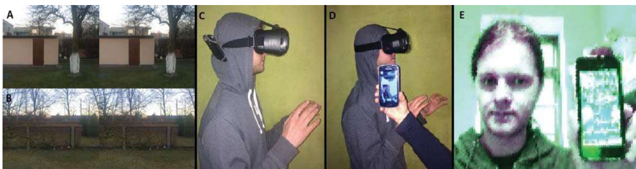
Fig. 1. Stereoscopic VR format video. A) front view, B) back view (second camera). ChameleonVR prototype: C) transmitter camera in the back of head, D) transmitter camera in the third-person perspective. E) aesthetic filter.
