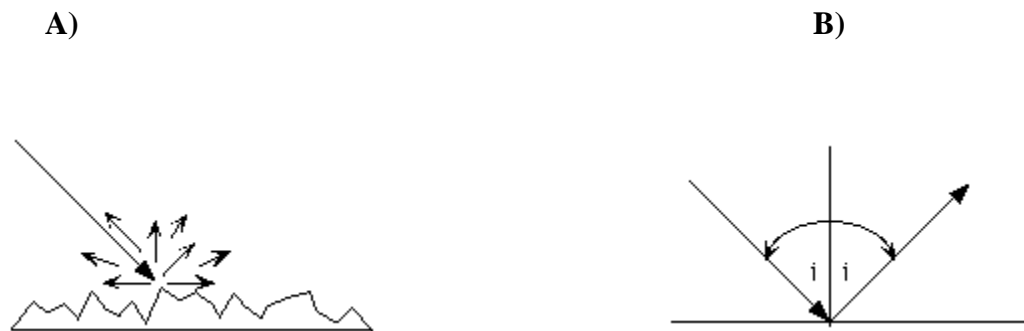
Figure 1. SAR signal scattering. A) A rough surface reflects most of the radar signal back to the receiving antenna, while a smooth surface (B) reflects the signal away from the receiving antenna. From Liew (2001).
