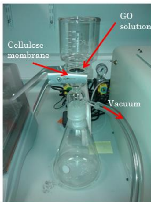
Figure 4.2: Vacuum filtration set-up. GO flake solution is filtered through a clamped cellulose membrane under vacuum.
