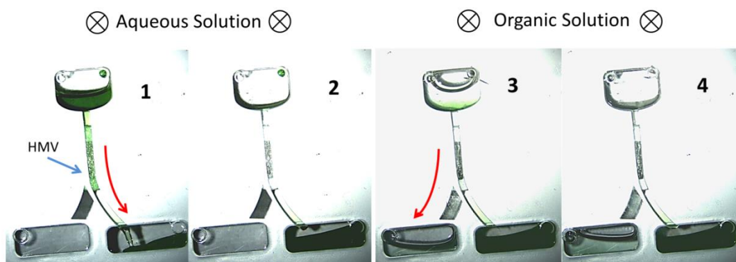
Figure 3.3: Routing of aqueous and organic flows using HM tab. The HM is impermeable to the aqueous phase. The fluid, therefore, travels over the 'closed' membrane and is collected in the right collection chamber (1, 2). The organic solution is loaded next; it passes through the 'open' membrane and is collected in the left collection chamber (3, 4). The centre of rotation is indicated above each image.
