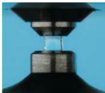
Figure 2.9: Droplet stretched on pedestal of Nanodrop spectrophotometer to give a 1 \text{ mm} pathlength. Adapted from Nanodrop Handbook (77).
