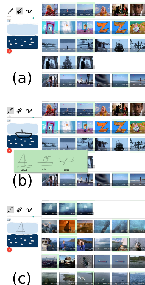
Figure 2: IMOTION QbS automcompletion in action: (a) user sketches a color sketch with the brush tool; matching images of the sea are retrieved (b) user switches to pencil and starts drawing a boat; a suggestion pop-up appears mid-sketch; (c) user selects the first option and the new results are displayed
