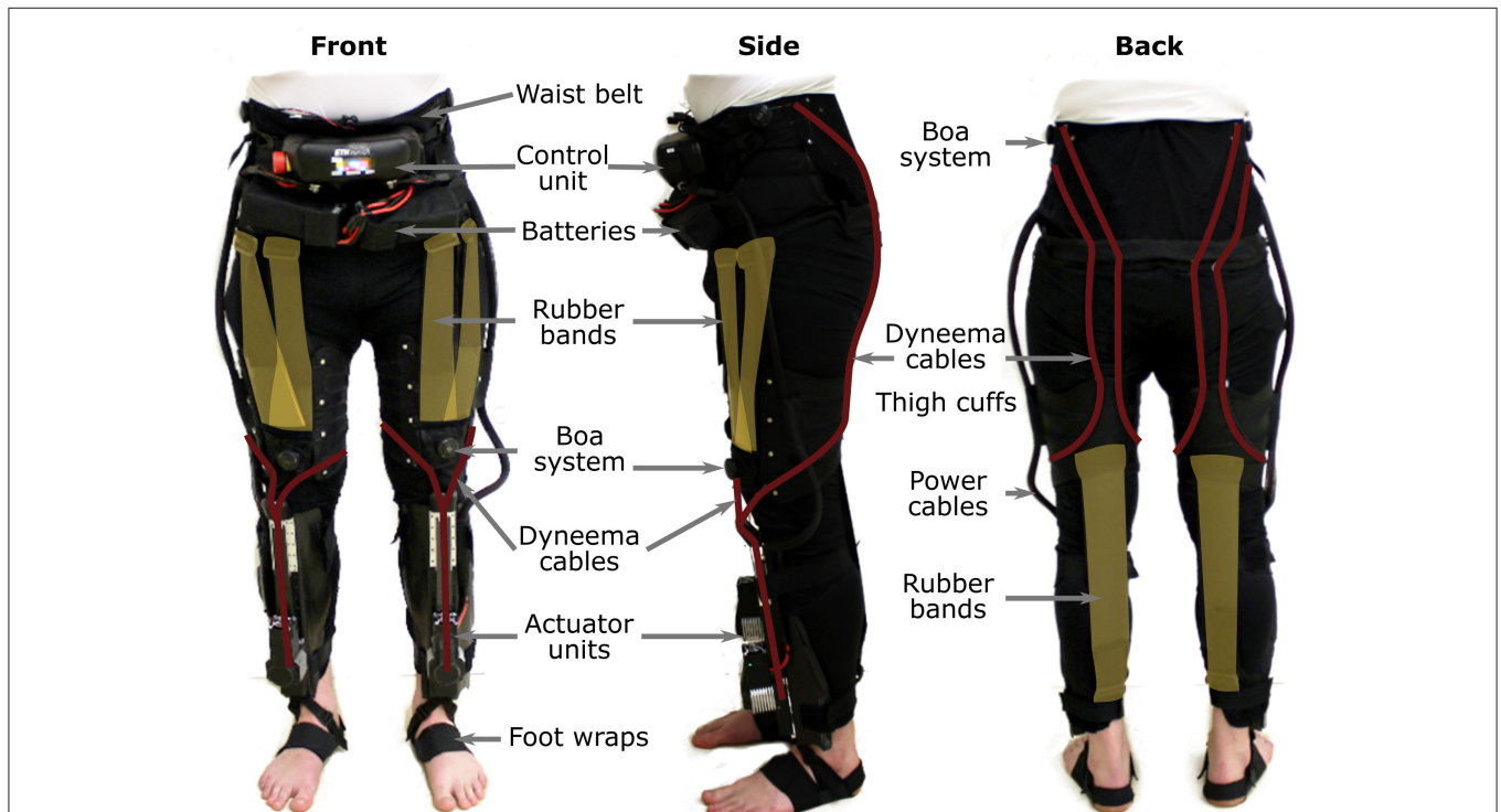
FIGURE 3 | The Myosuit resembles a pair of pants that include a waist belt and thigh cuffs sewn onto a stretchable base material. One set of rubber bands, designed to aid with hip flexion, attach at the front of the waist belt and the front of the thigh cuffs. A second set of rubber bands, designed to aid with knee flexion, attach at the back of thigh cuffs and the base of the actuation unit. The waist belt and thigh cuffs can be adjusted to the user's body to ensure proper fit of the device and efficient transmission of forces. The waist belt houses the control unit and a set of batteries used to power the actuator units. Power cords connect the control unit to the actuators and provide the required power for the system. Dyneema cables, routed along the garment layer, define the actuation path of the Myosuit.
