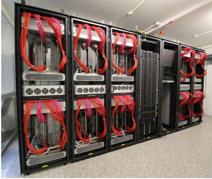
Figure 1.1: The BrainScaleS cluster in the European Neuromorphic Institute (ENI) in Heidelberg. In the first three and last two server racks are the BrainScaleS systems. Each rack offers space for four wafer modules.
