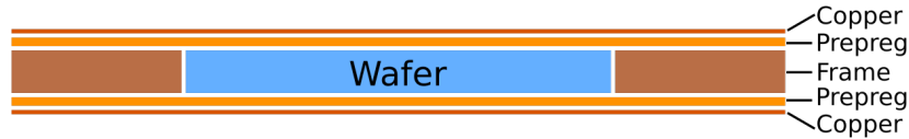
Figure 3.1: Generic stack up of the embedding process. The PCB layers are symmetrical added around the silicon wafer which is placed in the center of the stack up.
