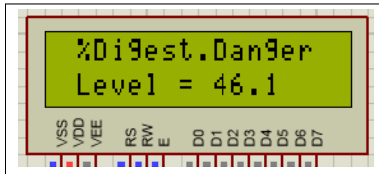
Fig. 6.14: Digester danger level LCD reading
