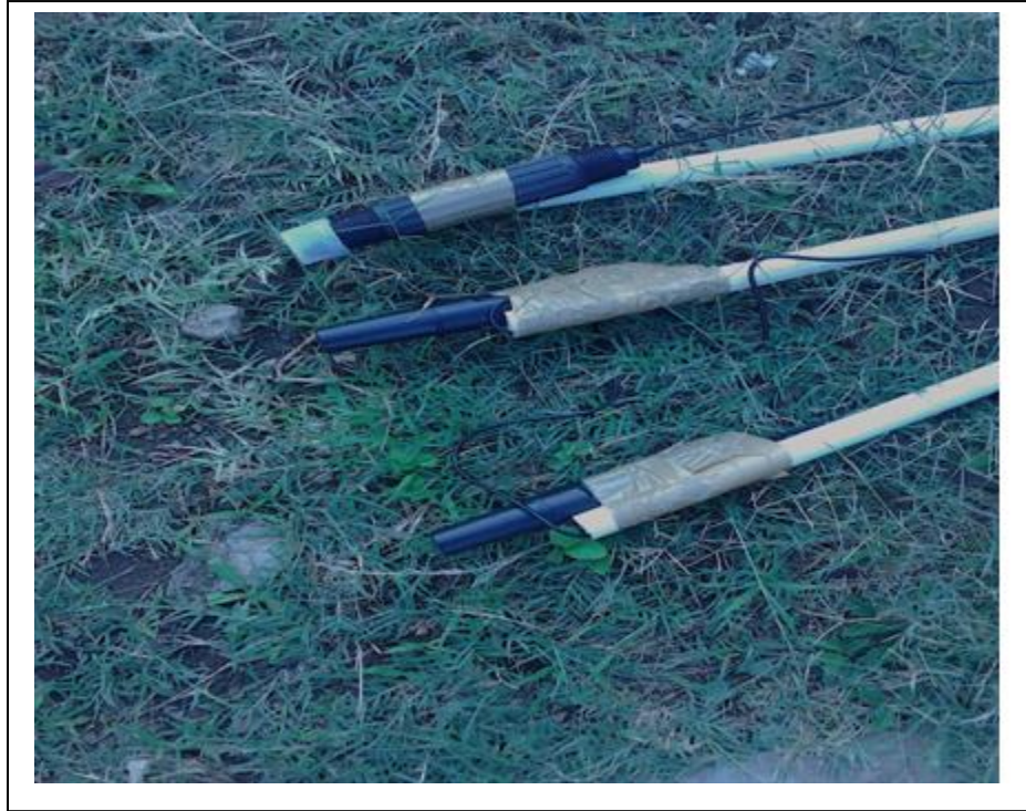
Fig. H.4: pH, redox and electrical conductivity sensors mounted on 6m 19mm PVC conduits
