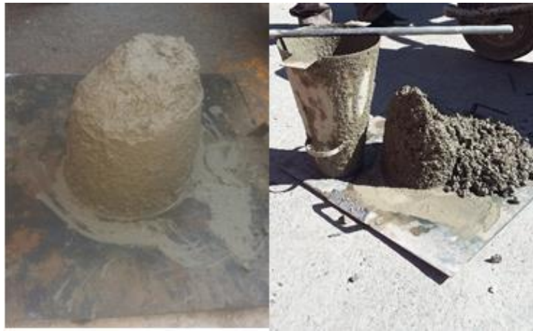
Fig. 4 –Slump test of concrete for control (left) and 70% glass (right)
