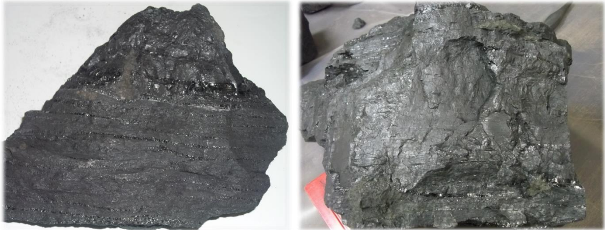
Figure 1: Coal Samples with mineral matter and different maceral compositions.
