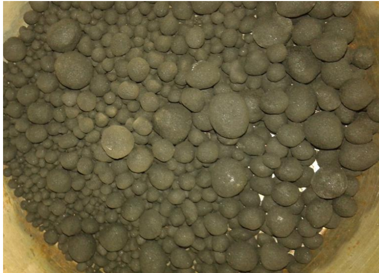
Figure 6: Pellets produced from the laboratory experiments using the different binders.
