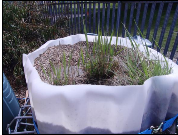
Fig. 2. An overhead photo of the prototype wetland at the Nottingham Trent University. The basis of the module was an IBC container.
