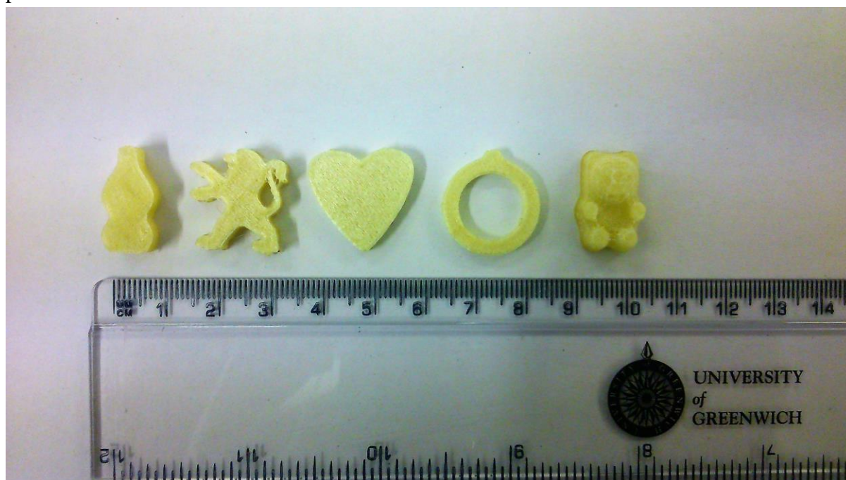
Fig. 1: Photographic image of the 3D printed medicines loaded with IND as model substance
