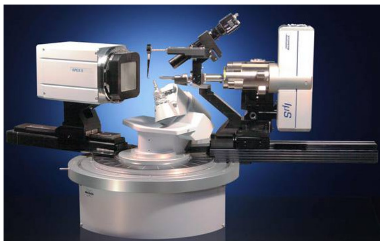
Figure 2.2: Photograph of a typical single crystal diffraction instrument, with the source shown at right and the detector left. The position of the detector is rotated around the goniometer to collect a hemisphere of data.
