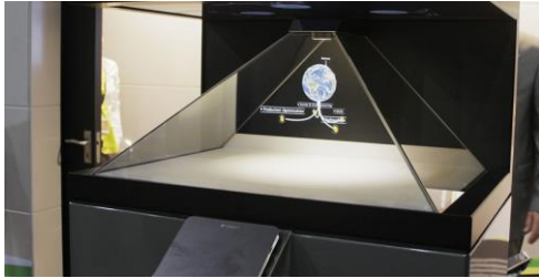
Figure 1 A reflective prism display [3]. A flat screen is placed on top of the prism as an image projector
