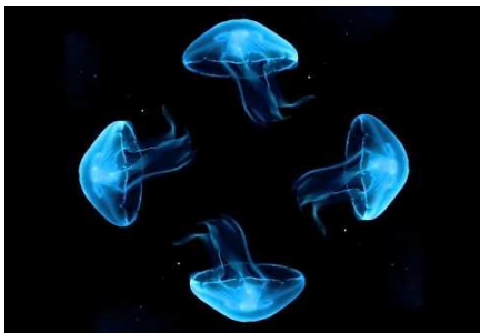
Figure 2 The four viewports with images of a jellyfish as the viewport content. This final image is ready to be projected by an image projector onto the front, back, left, and right side of the prism [16],
