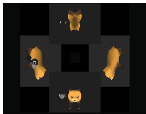
Figure 6 Simply using four cameras without adjusting camera variables create an obstructive view on the viewports in the Game window
