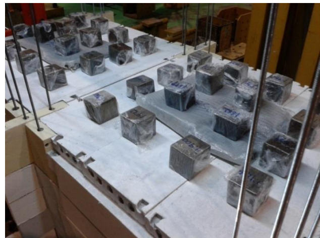
Figure 8 First floor slabs and live loads
