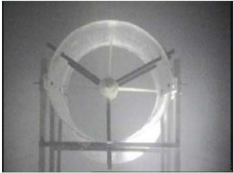
Figure 8. Augmented Diffuser HAMCT device through observations
