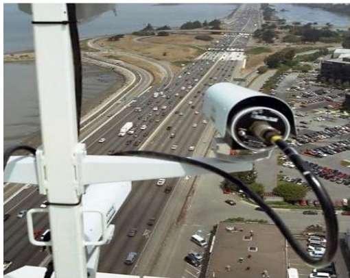
Figure 2 Camera fitted to a high place by Next Generation Simulation Program (NGSIM) data collection site [49].
