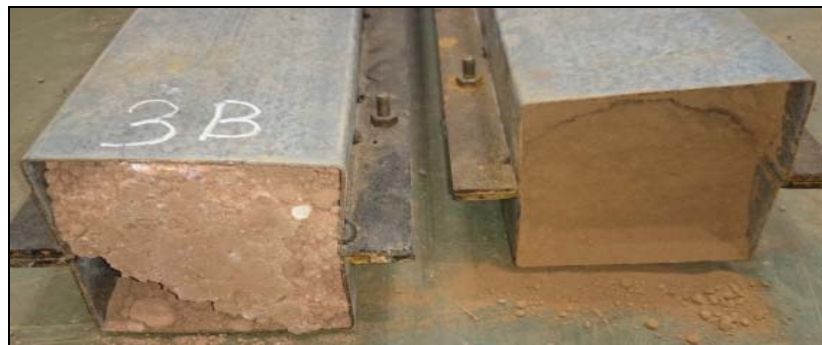
Figure-8. The failure of the compacted soil after the test is completed.
