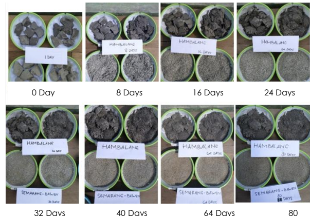
Figure 9 Disintegration of Hambalang and Semarang-Bawen clay shale up to 80 days due to wetting drying process twice soaked in every 8 days
