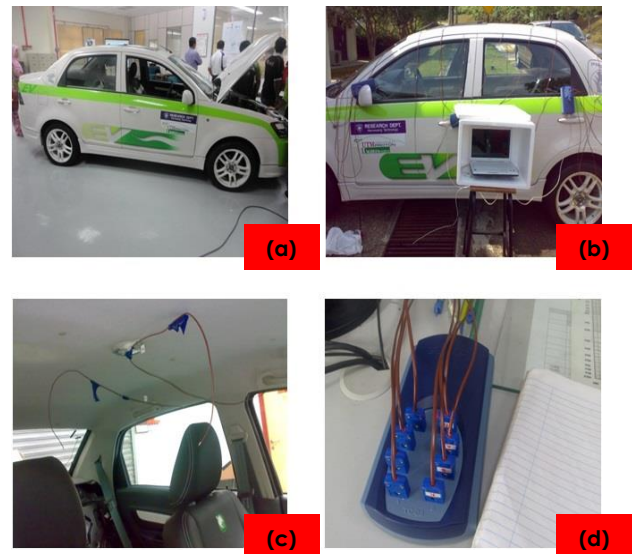
Figure 2 (a) The Proton Saga car, (b) The data acquisition system, (c) Additional thermocouples to measure air temperature at the front and rear section of the passenger compartment, (d) The TC-08 USB data logger
