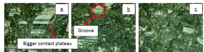
Figure 5 Surface topography at 15 bar and 60 rpm in presence of road particle (a) left, (b) middle, (c) right of pad
