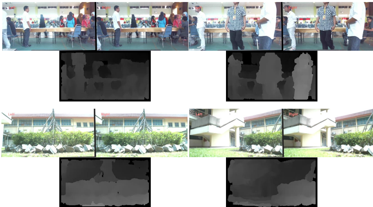
Figure 6 At the top, the pair images captured by robot stereo cameras, at the bottom, the disparity map calculated by the proposed algorithm after noise removal and edge normalization in non-ideal outdoor and indoor lighting conditions
