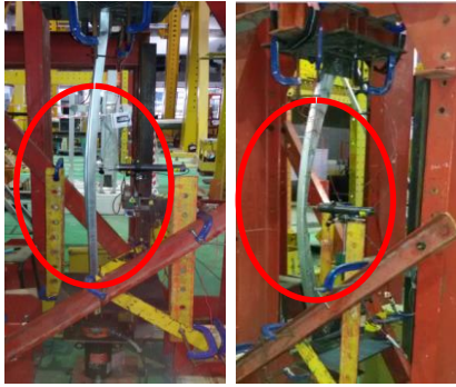
Figure 6 The failure mode of global buckling for normal and cut-curved section
