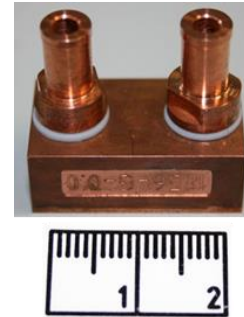
Figure 1 Tested microcooler with structured area
