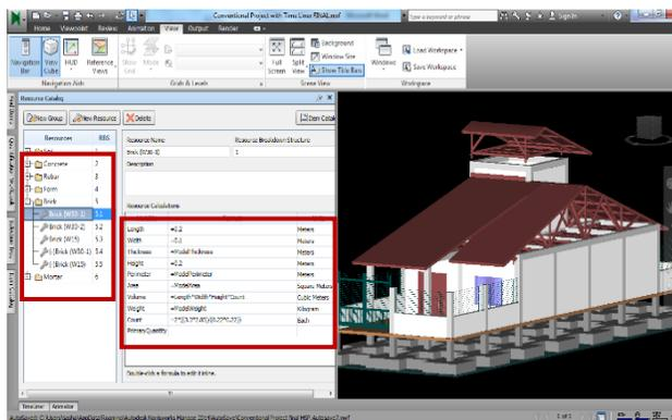
Figure 4 Identification of Materials in Navisworks Manage 2014
