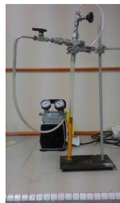
Figure 3 Vacuum deposition setup for catalyst deposition
