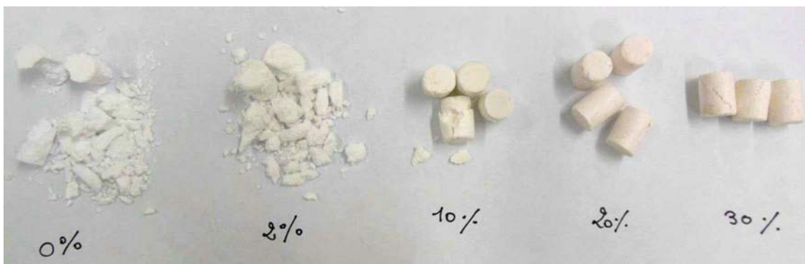
Fig. 5 Photographs of the wet composite cement blocks, including various amounts of CMC, after the compressive test
