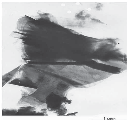
Fig. 5. Electron micrograph of a sample of untreated vermiculite of fired T = 400^{\circ} \text{C} .
